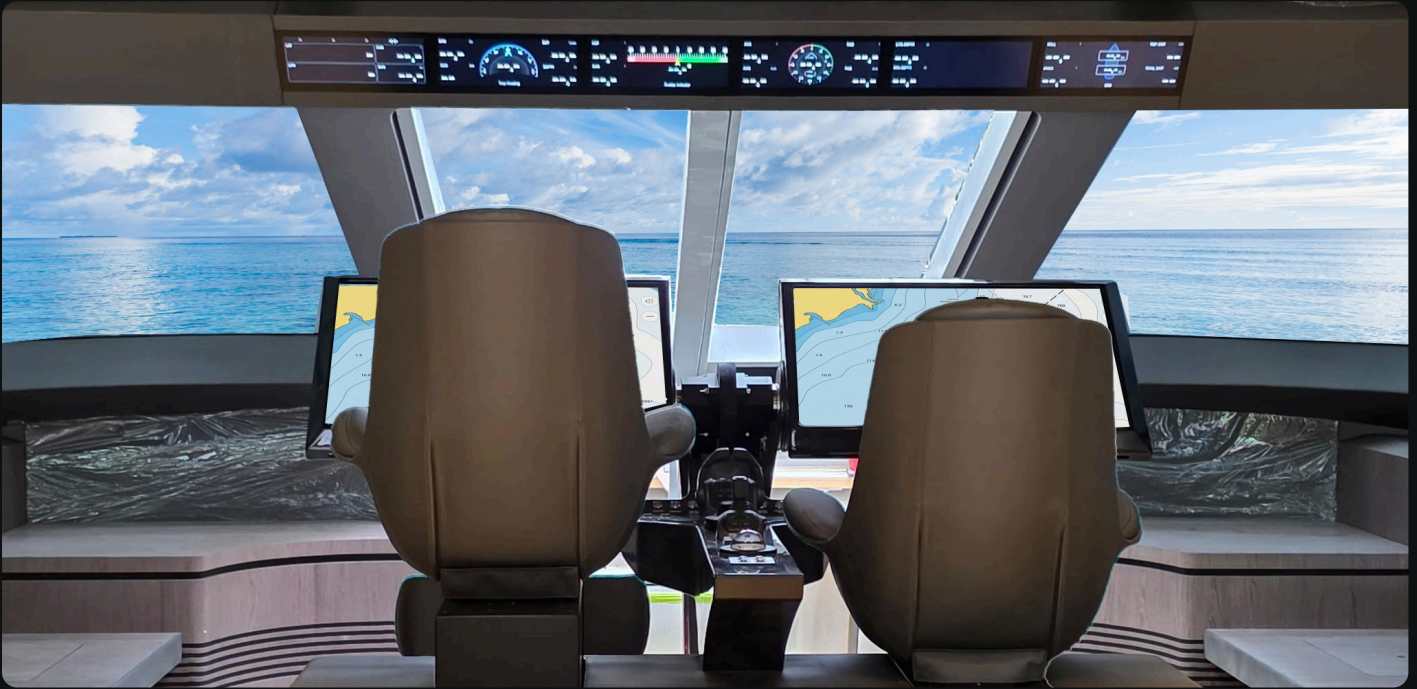
McConaghy MC86GT helm. Unified displays and 300 digital switching points on an 86 ft power catamaran.
